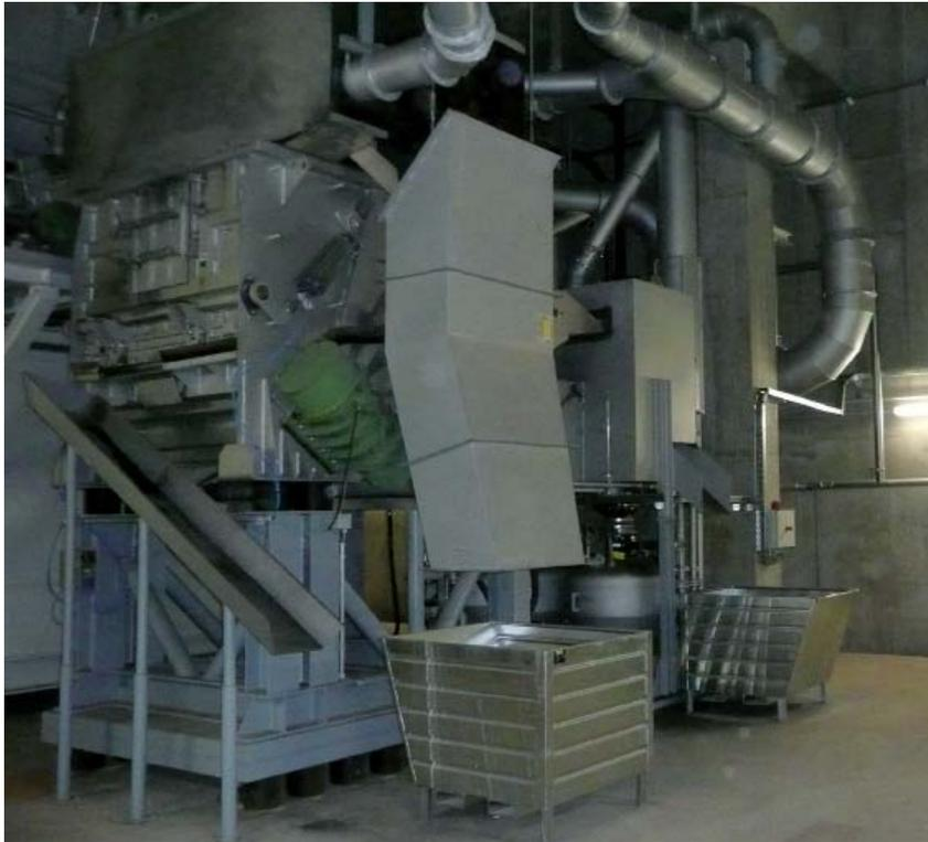
**Figure 2:** Shakeout and crushing station with two vibratory lump crushers (output: 2 x 25 t/h)
