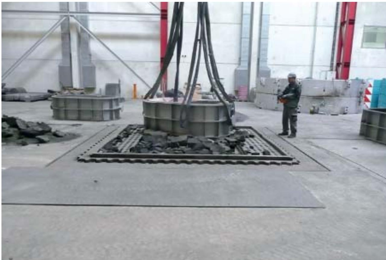
4.2 x 4.2 m shakeout grid with a total load of 50 t (Photos: F.A.T.)
