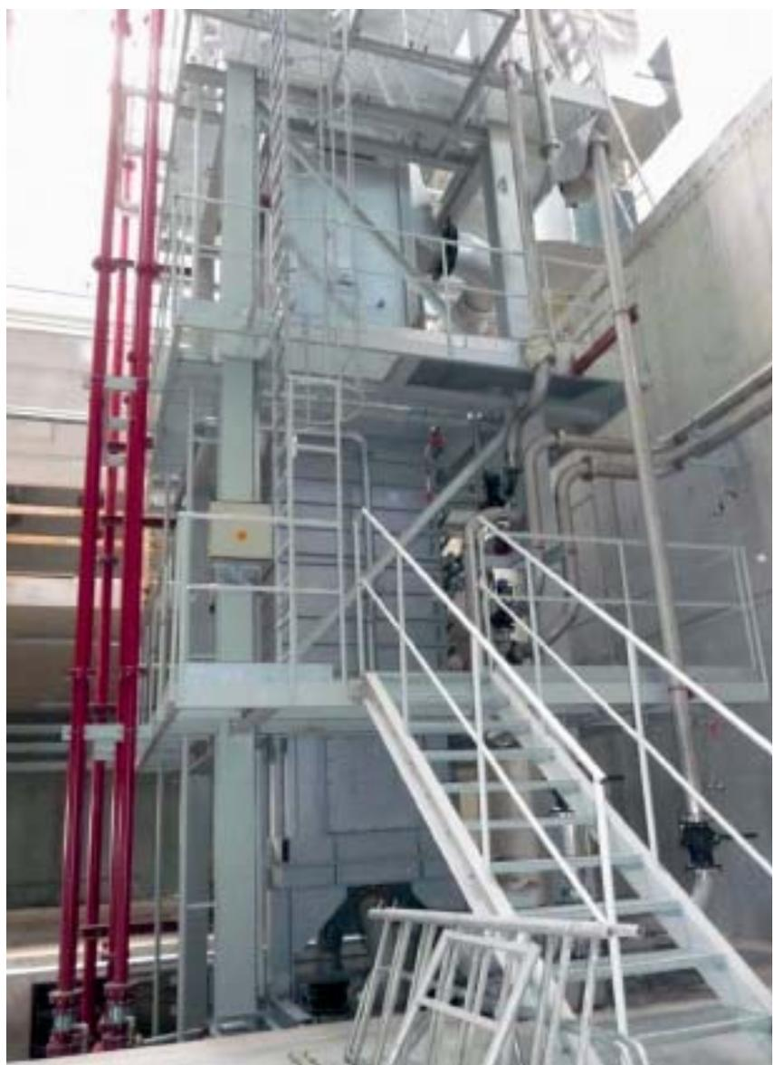
Figure 1: F.A.T. sand reclamation system with sifter and reflux cooler (output: 50 t/h)
