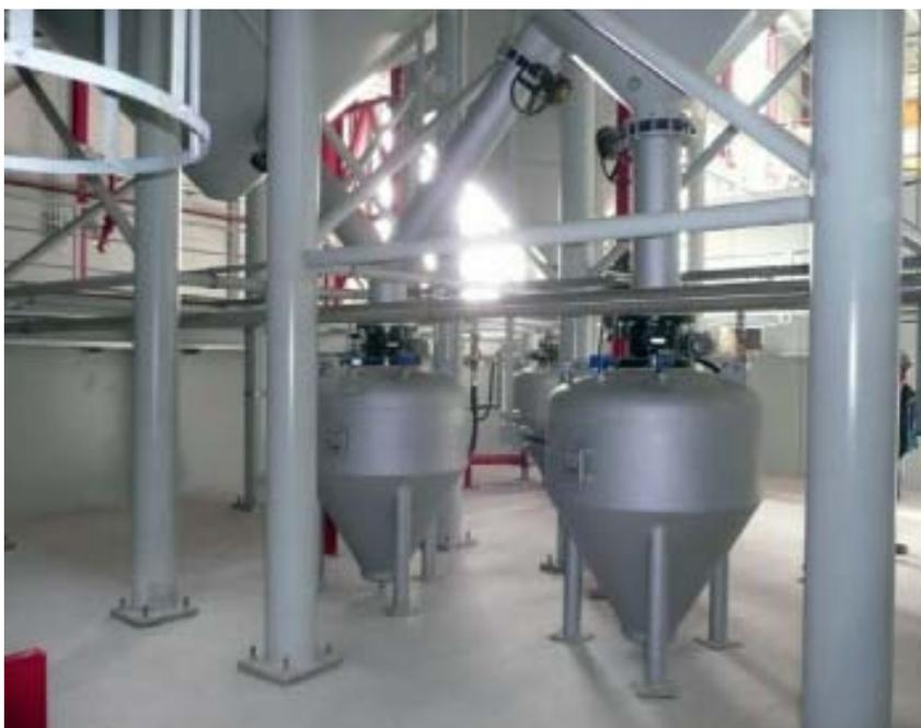
**Figure 3:** Pneumatic sand supply with F.A.T. shuffle-type conveyors
